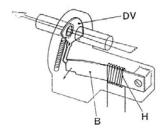
Fig.1A Extra air valve (cold)
